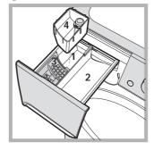
This function is particularly useful for the removal of stubborn stains. Insert extra compartment 4 (supplied with the appliance) into compartment 1. When pouring in the bleach, be careful not to exceed the "max" level marked on the central pivot (see figure). To bleach laundry with no other
